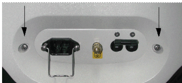
Figure 8-7 Rear Cover Screws in AC Input Box Unit
