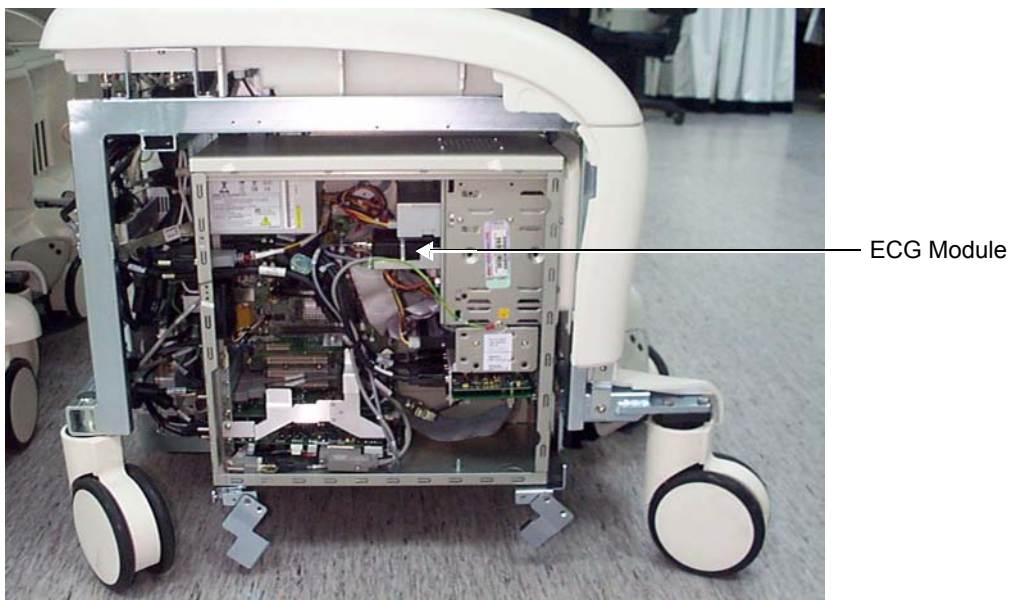
Figure 8-71 ECG Module - BEP2
