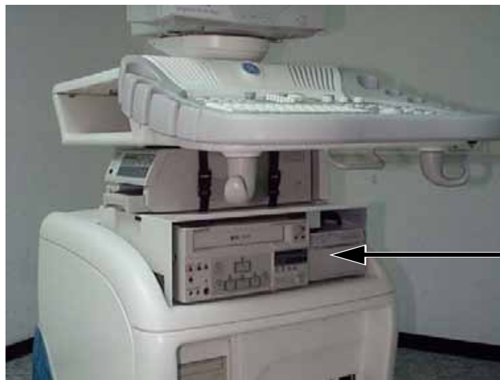
Figure 8-109 B/W Video Printer Installed in the Vivid™ 3 (Configuration with UP21MD Printer)
