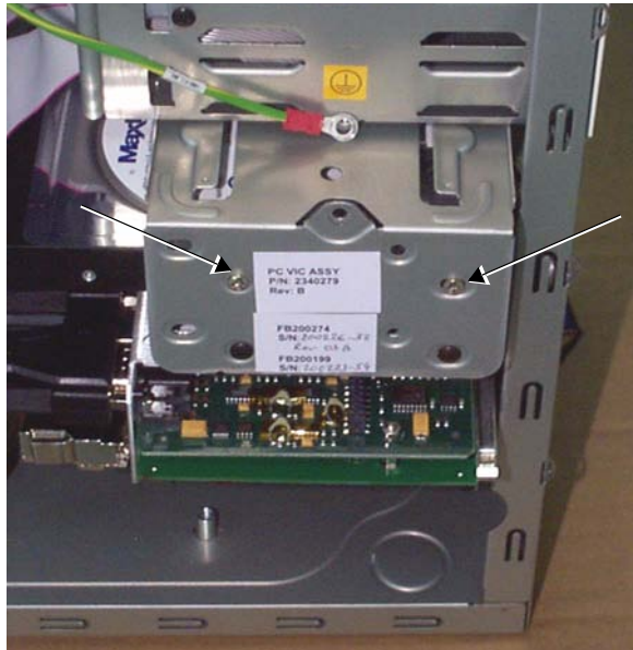
Figure 8-85 Hard Disk Removal 2
