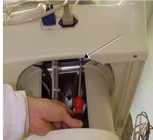
Figure 8-19 Removing Screws from the AC/VGA Connectors Box
