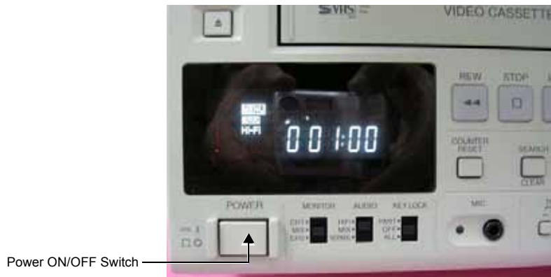
Figure 8-116 Mitsubishi VCR Front Panel - Power Switch
