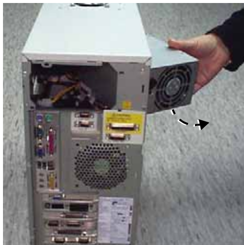
Figure 8-81 Removing the BEP2 Power Supply with Cable Loom and Connectors
