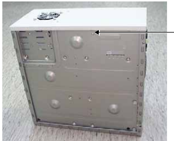
Figure 8-76 BEP2 with Side Cover Removed
