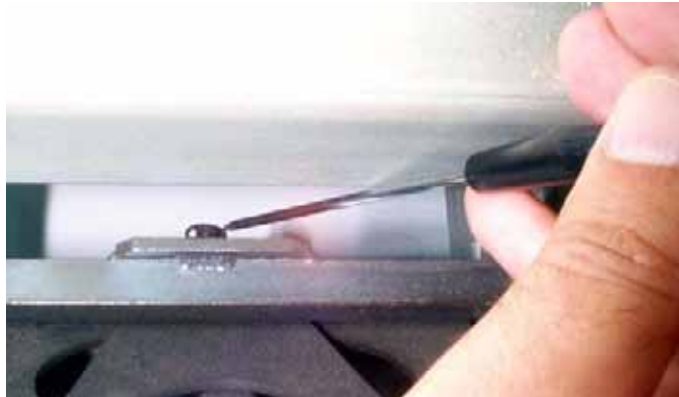
Figure 8-100 Releasing the Spring Washer from the Center of the Transverse Arm
