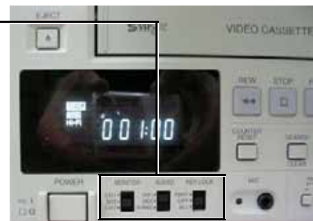
Figure 8-125 Mitsubishi VCR - Switches Settings (Front Panel)
