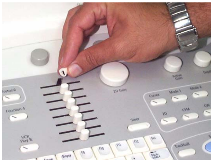
Figure 8-38 ATGC Slider Keycap Replacement
