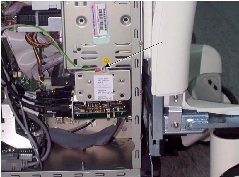
Figure 8-84 Hard Disk Removal 1
