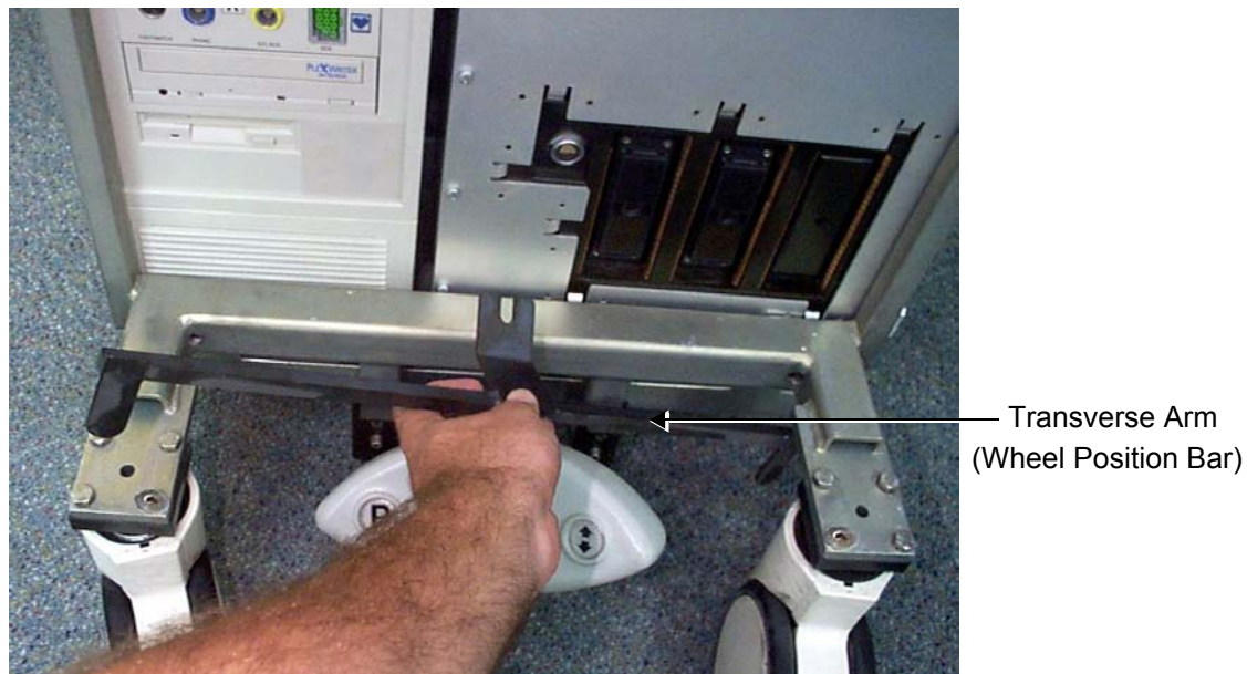
Figure 8-103 Removing the Transverse Arm
