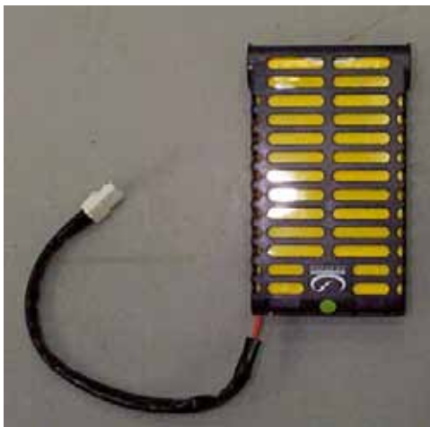
Figure 8-64 Plug & Scan Battery Removed
