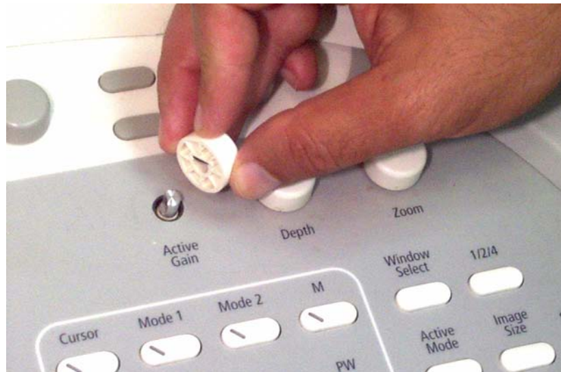
Figure 8-39 Rotary Knob Replacement
