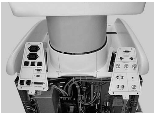
Figure 8-13 Connector Panels - Loosened
