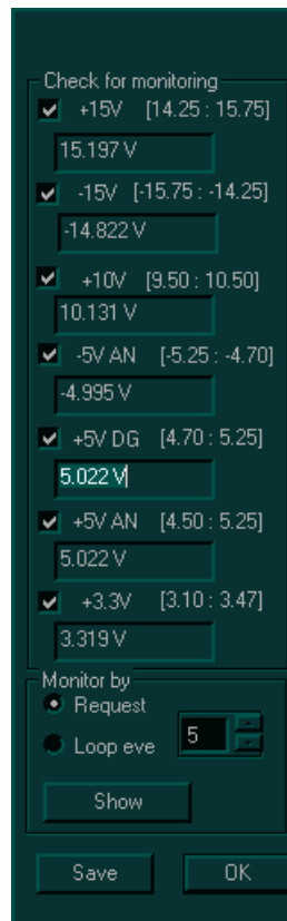
Figure 7-38 LVPS Voltage Ranges
