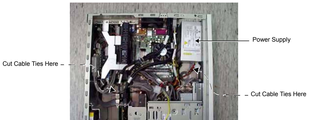
Figure 8-78 BEP2 Power Supply and Cable Ties
