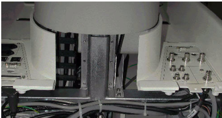
Figure 8-12 Top Cover with Collar Removed
