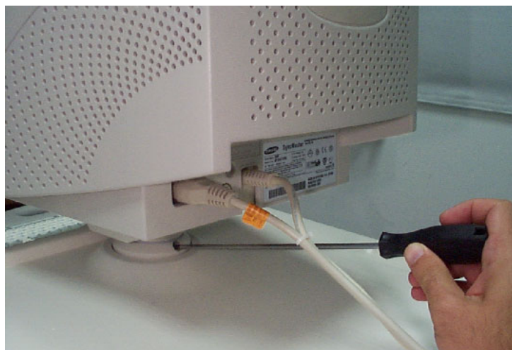
Figure 8-30 Releasing Screw at Base of 17" Monitor
