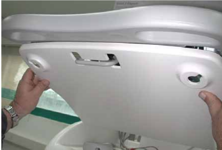
Figure 8-16 Removing the Bottom Keyboard Cover
