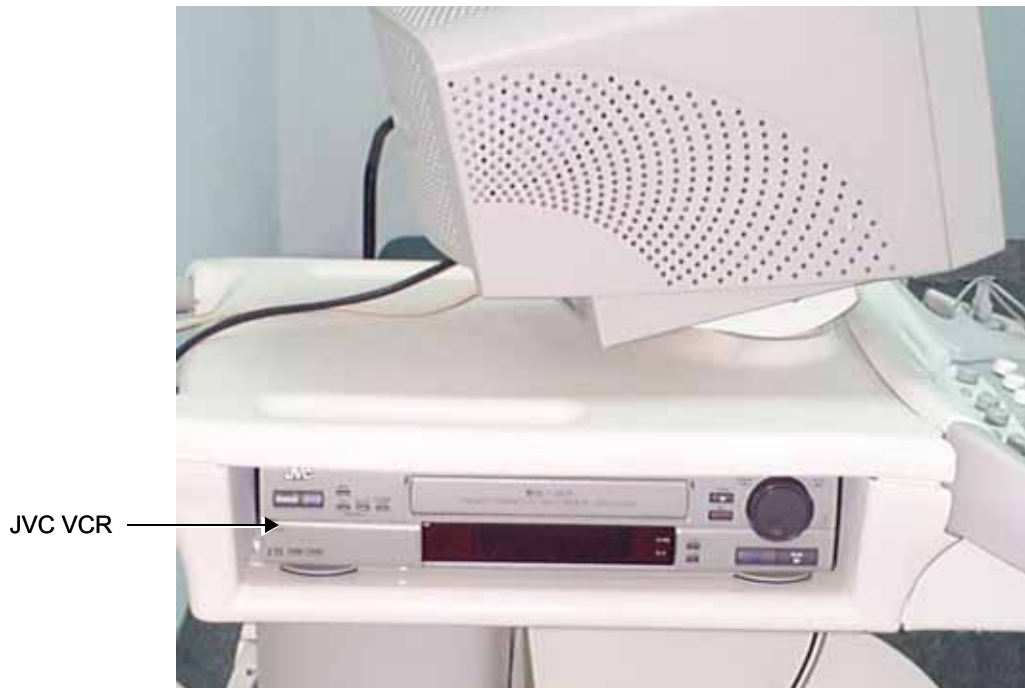
Figure 8-141 JVC VCR Installed in Compartment
