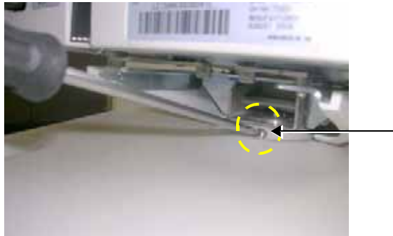
Figure 8-28 Releasing Screw at Base of Samsung 15" Monitor
