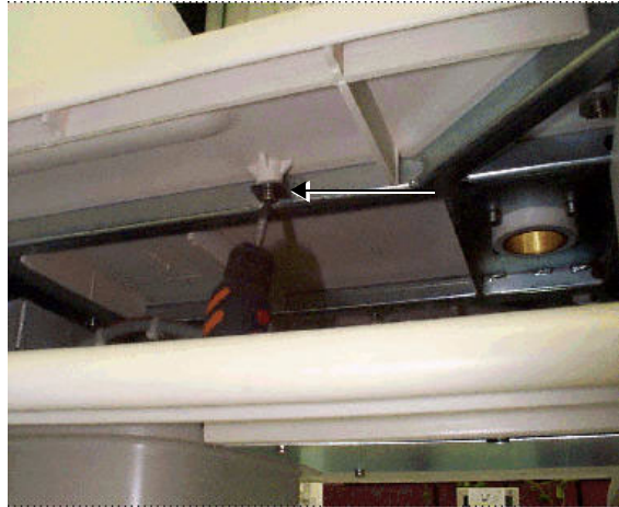
Figure 8-22 Removing Top Cover Screws (2)
