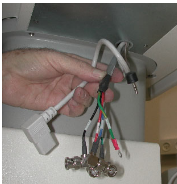
Figure 8-169 Color Printer Cables through Metal Bottom Cover Slot
