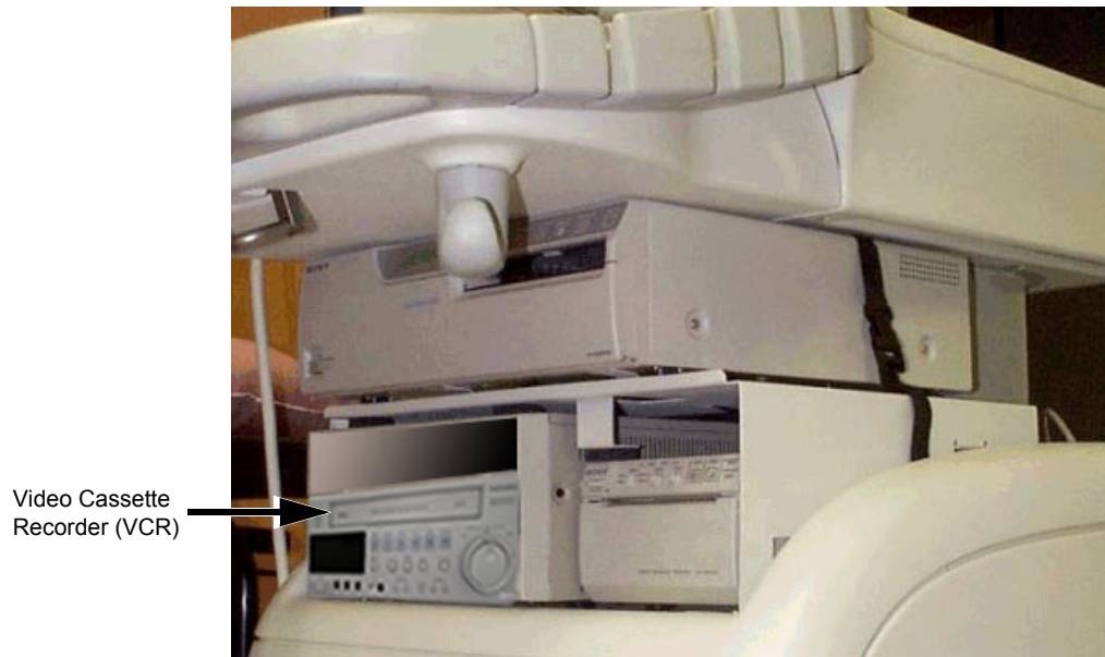
Figure 8-113 Video Cassette Recorder (VCR) Installed in the Vivid™ 3 Ultrasound Unit Configuration with UP2950 Printer
