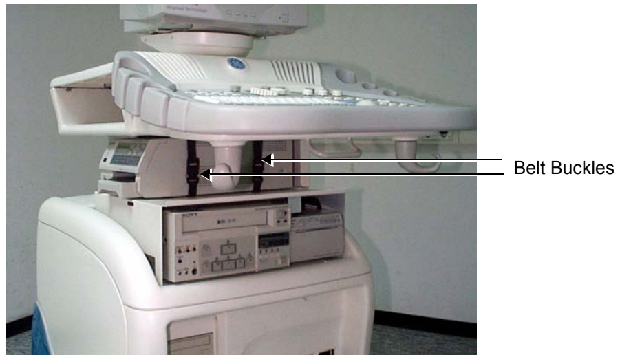
Figure 8-176 Belt Buckles Securing Printer
