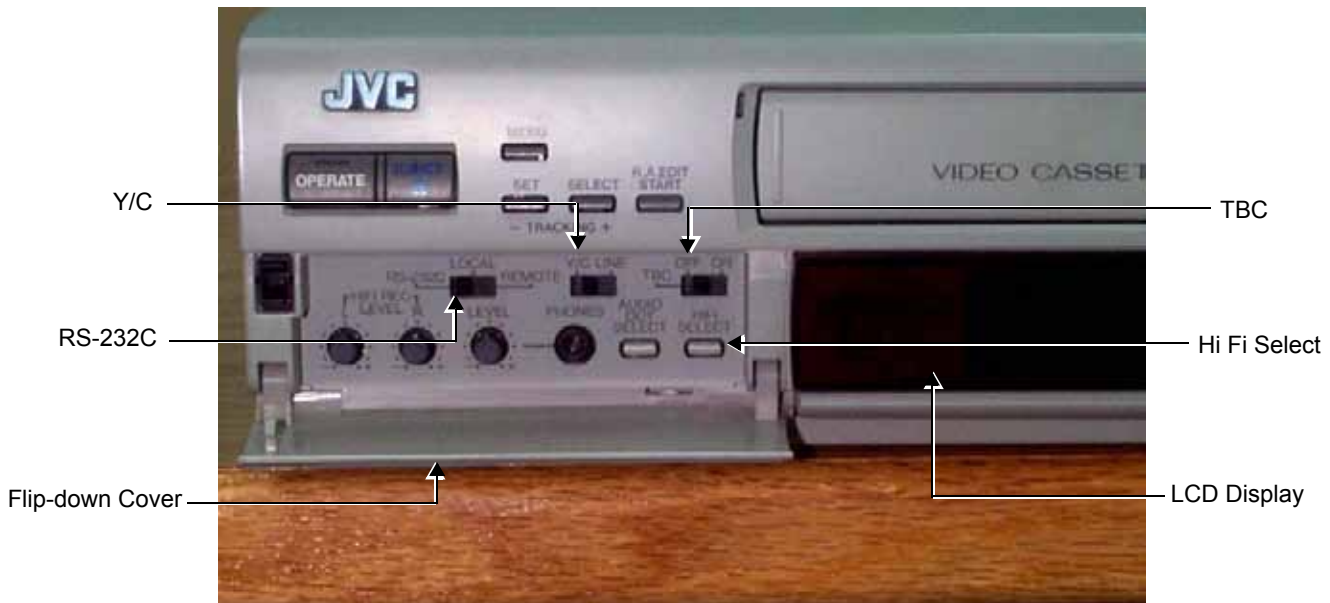
Figure 8-133 JVC VCR Front Panel - Switch Settings
