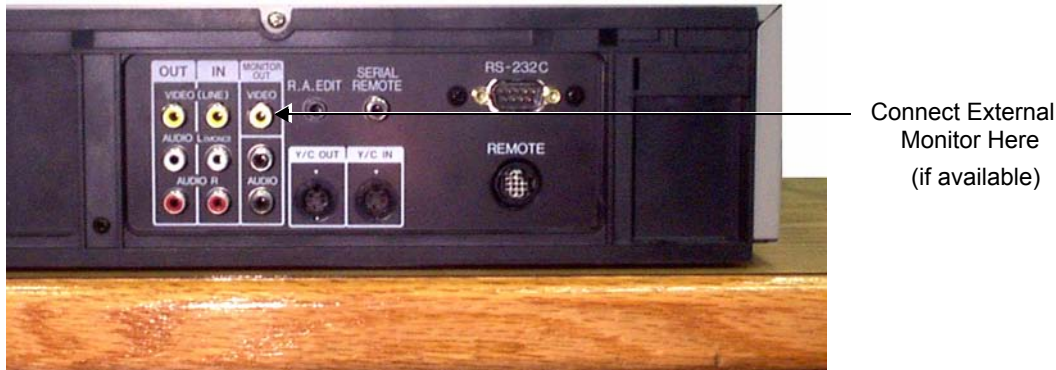
Figure 8-134 JVC VCR - Rear Panel - External Monitor Connection
