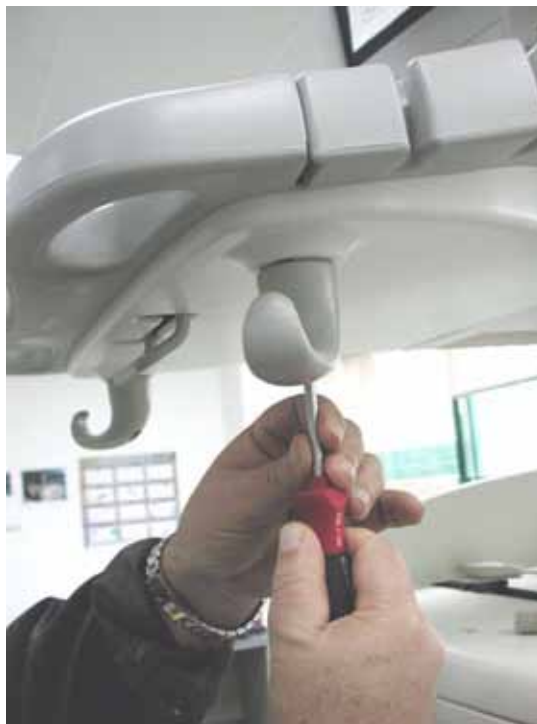
Figure 8-15 Removing Probe Cable Hooks under Keyboard Cover
