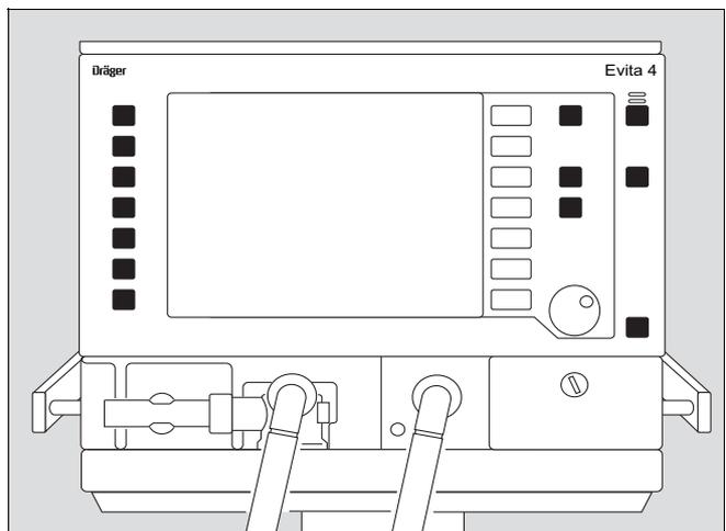
The keys for routine functions are placed to the right and left on the outside of the front panel. Frequently used function keys are placed on the right, e. g. the key »
