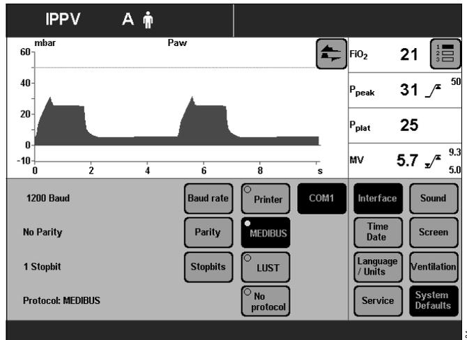
To connect a printer to Evita 4 (HP Deskjet 500 and compatible printers with serial interface).
