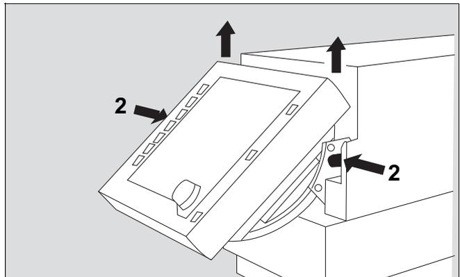
3 Lock it into position = pull tab under the holder down and turn it towards the wall rail.
