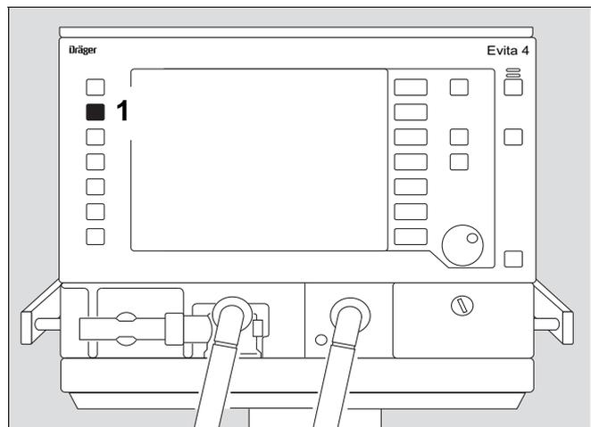
Evita 4 ventilates the patient in the set ventilation mode with increased O<sub>2</sub> concentration: 100 % O<sub>2</sub> by volume in adult mode, and 25 % higher O<sub>2</sub> concentration than the set value in paediatric mode.
