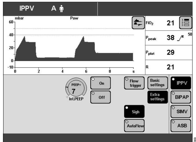
**AutoFlow**<sup>®</sup> – for automatic regulation of the inspiration flow. With AutoFlow\*, the inspiration flow is decelerated and regulated, so that at the selected tidal volume V<sub>T</sub> with the current lung compliance a minimum airway pressure is reached and pressure peaks are avoided.
