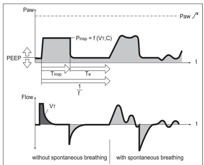
This effect can also be caused during ventilation, e. g. due to a build-up of secretion. In this situation, the pressure is limited by the alarm limit »Paw  $\sqrt{\wedge}$ «. The pressure rise stops 5 mbar below the alarm limit »Paw  $\sqrt{\wedge}$ « and the alarm »Volume not constant !!« is only given when the set tidal volume  $V_T$  is not longer applied.
