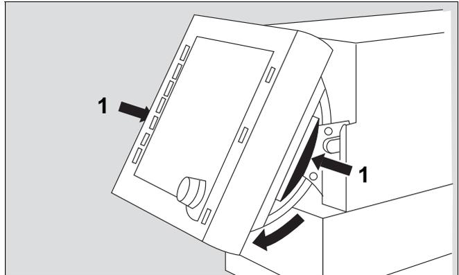
2 Press and hold the unlocking buttons on the right and left, lifting the control unit out of the mount on the Evita 4 at the same time.
