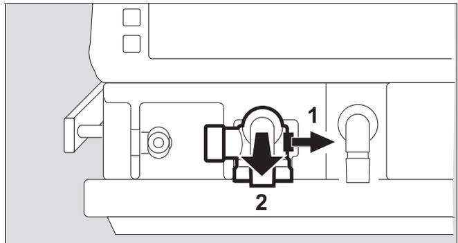
If the expiration valve is fitted with an optional water trap:
