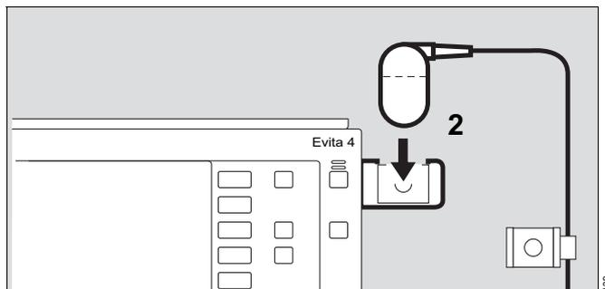
**Performing CO<sub>2</sub> zero calibration when using disposable cuvettes**
